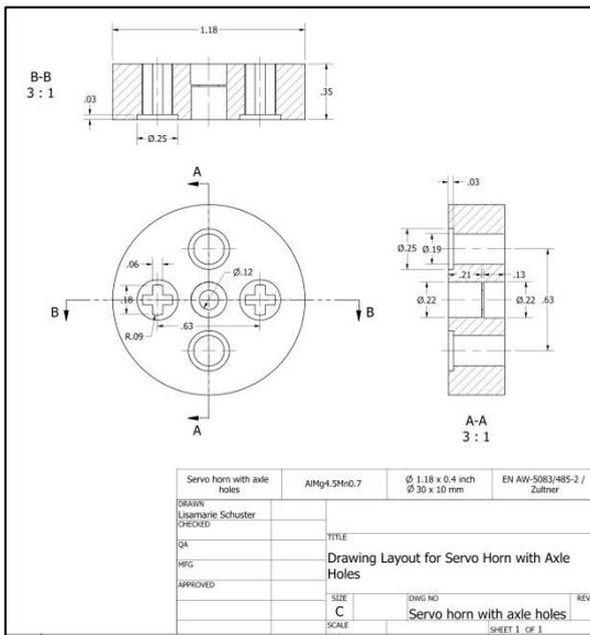
**Figure 5.** New designed Lego compatible servo horn
