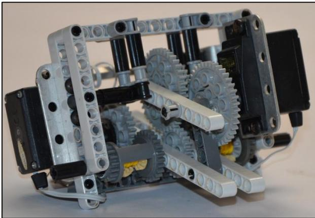
**Figure 7.** Experimental 3-motor-drivetrain
