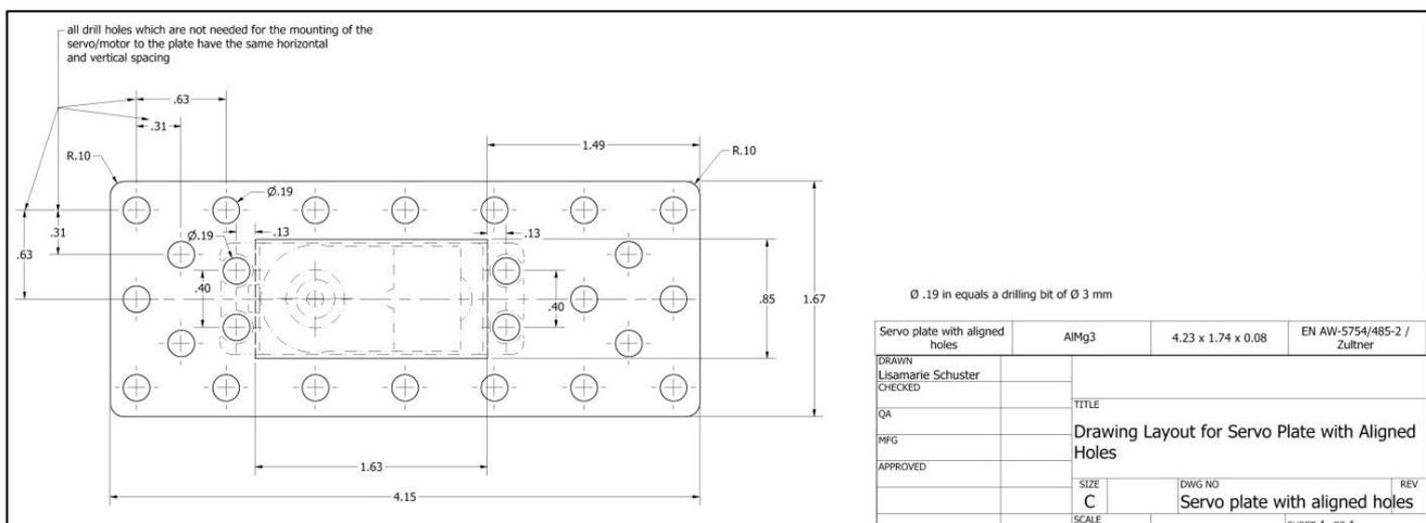
**Figure 4.** Dimensions of the new designed servo plate
