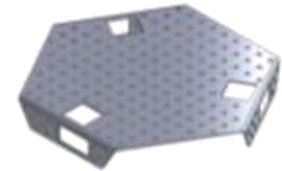
Fig. 4. Wallaby Base for Omni-wheels [4]
