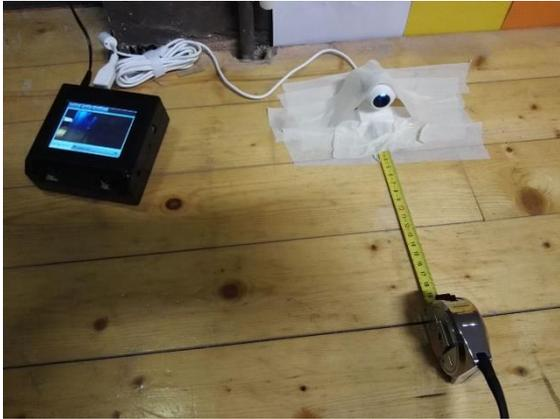
The objects used consistently had an area of 15cm by 7cm. We used different colours in a setting of artificial light provided by neon lights.
