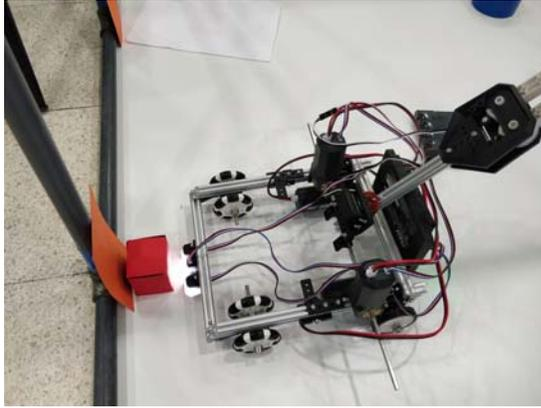
Fig 7. Robot moving closer to the object to detect colour.
