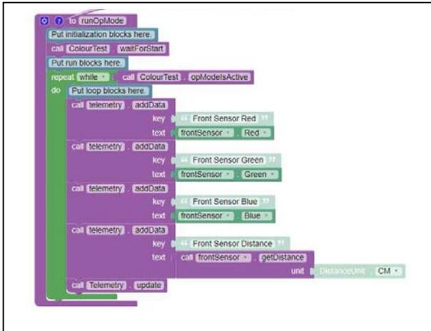
Fig 8 Screenshot for the code in Blockly to control the colour sensor
