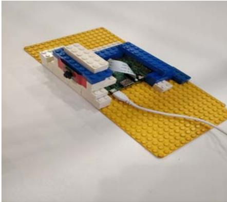
Fig. 3. The PI Camera and RPi set up in a Lego Structure to keep a steady position
